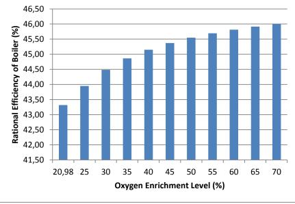
Fig. 4 Rational efficiency of the boiler at different oxygen enrichment levels Table 1 Irreversibility for different oxygen enrichment levels
