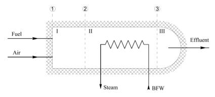
Fig.1 Scheme of a coal fired steam boiler
