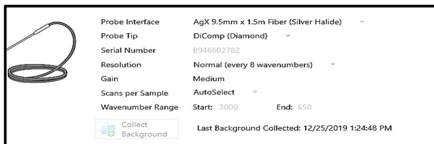
Figure 2. The IC IR 7.1 program interface, collecting environmental background in the reactor
