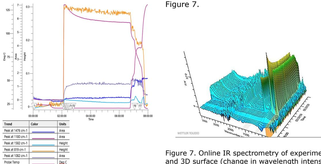
Figure 7. Online IR spectrometry of experiment 2 (left) and 3D surface (change in wavelength intensity over time) of online IR spectrometry (right)
