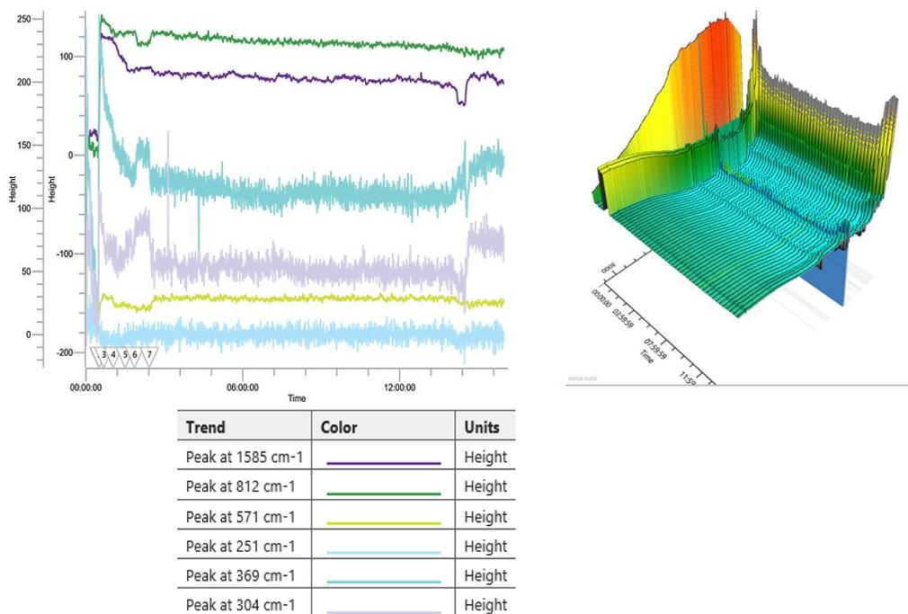
Figure 11. Online Raman spectroscopy of experiment 4 (left) and 3D surface of online Raman spectroscopy (right)
