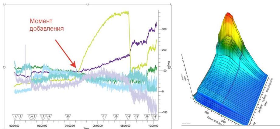
Figure 12. Online Raman spectroscopy (left) and 3D surface of online Raman spectroscopy (right) for experiment 4 after 5 grams of premade MDI addition
