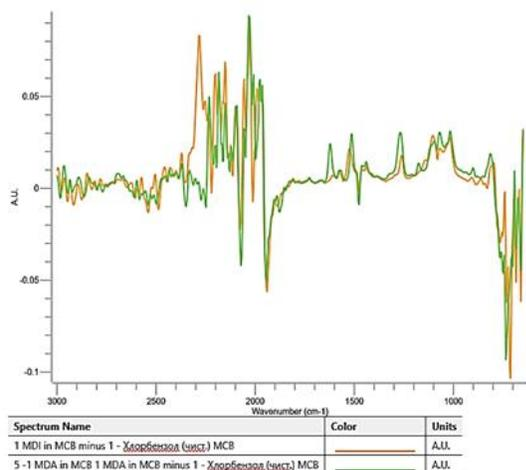
Identification of MDI and MDA can be accomplished by subtracting chlorobenzene spectra from solutions spectra and determining characteristic wavelengths for MDA and MDI (Figure 4). These wavelengths can be used for online IR spectrometry.
