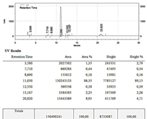
Figure 6. HPLC data for 1,5 specimens for experiment 1
