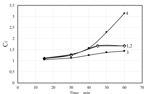
Fig. 4 Kinetics of MCTP foaming at the ratio MCTP:CBA = 100:5 (wt. part) at T = 150°C depending on the modifier PVC amount (wt. p./100 wt. p. of CTP): 1) - 3; 2) - 7; 3) - 10; 4) - 20
