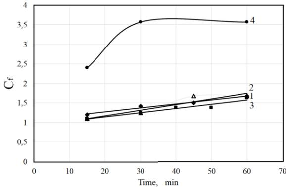
Fig. 5 Kinetics of the MCTP foaming at the ratio MCTP:CBA = 100:3 (wt. part) at T = 150°C depending on the modifier PVC amount (wt. p./100 wt. p. of CTP): 1) - 3; 2) - 7; 3) - 10; 4) - 20.
