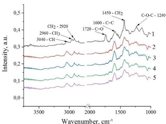
Fig.8. FTIR-spectra of the initial CTP (1), foamed CTP (2) and MCTP solid foams (CBA amount 5 wt. p./100 wt. p. of MCTP). The composition of solid foams based on the MCTP (PVC amount, wt. p./100 wt. p. of CTP): 3) - 5; 4) - 10; 5) - 20
