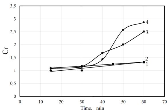
Fig. 3 Kinetics of the MCTP foaming at the ratio MCTP:CBA = 100:1 (wt. part) at T = 150°C depending on the modifier PVC amount (wt. p./100 wt. p. of CTP): 1) - 3; 2) - 7; 3) - 10; 4) - 20
