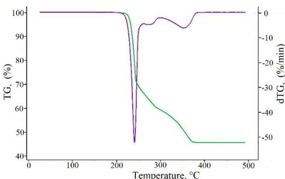
Fig. 1. Thermogravimetric curves of ADCA
