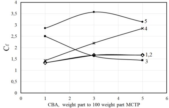
Fig.6 Dependence of the maximum foaming criterion value ( $C_{max}$ ) for the MCTP on the CBA amount at T=150°C and the holding time of 60 minutes. MCTP with PVC content (wt. p./100 wt. p. of CTP): 1) - 3; 2) - 7; 3) - 10; 4) - 15; 5) - 20.
