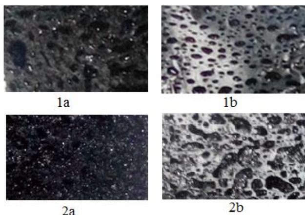
Fig.7 Photographs of gas-filled MCTP samples (3 wt. part of CBA per 100 wt. part MCTP): a - pores inside the sample; b - pores on the surface of the sample. MCTP samples (wt. part of PVC per 100 wt. part of CTP): 1) 10; 2) 20
