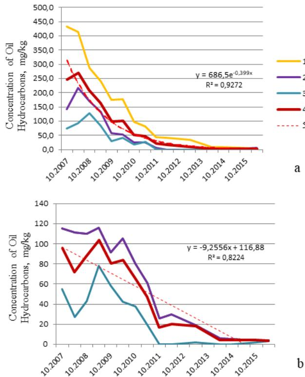
Fig. 3. The dynamics of the change in the concentration of oil products in various parts of the research site in the interval of 0.1-0.2 m (a) and in the interval of 0.3-0.5 m (b): 1 – the silts of the elementary transsuperaqual landscape, 2 – the soils of the elementary downslope (transeluvial) landscape, 3 – the soils of elementary autonomous eluvial landscape, 4 – the soils and silts of the entire research area, 5 – trend line for the graph of the change in the average content of the OP
