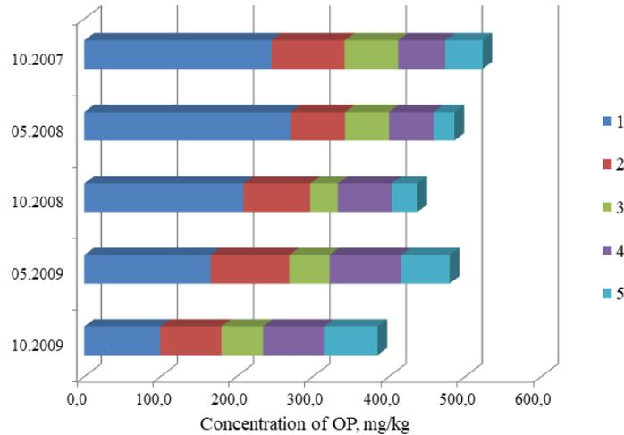
Fig. 2. Dynamics of changes in the average concentration of oil products in soils with depth and time. Sampling intervals, m: 1 – 0.1-0.2, 2 – 0.3-0.5, 3 – 0.8-1.0, 4 – 1.3-1.5, 5 – 1.8-2.0.
