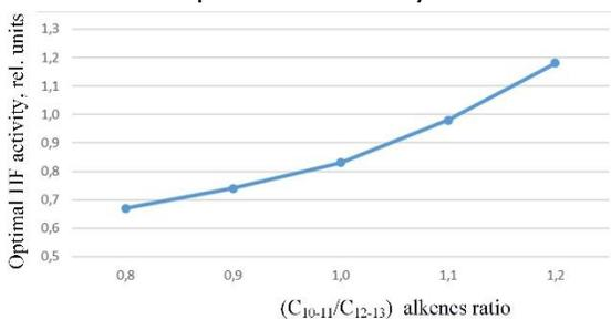
Fig. 5. Effect of feed composition on catalyst performance
