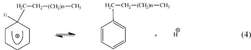
Figure 1. Mechanism of benzene alkylation with alkanes
