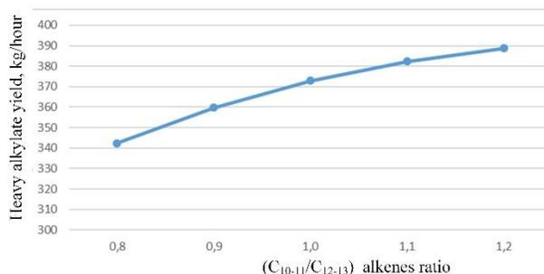
Figure 4. Yield of heavy alkylate depending on the ( $C_{10-11}/C_{12-13}$ ) alkenes ratio
