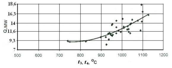
Figure 6. The dependence of the generated heat amount on the temperature in zones 3 and 4
