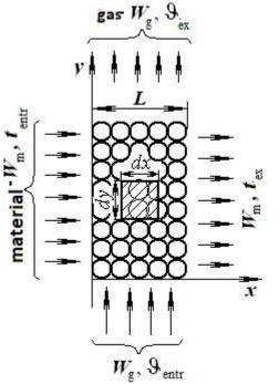
Figure 2. Scheme of heat exchange process in the layer of lump material
