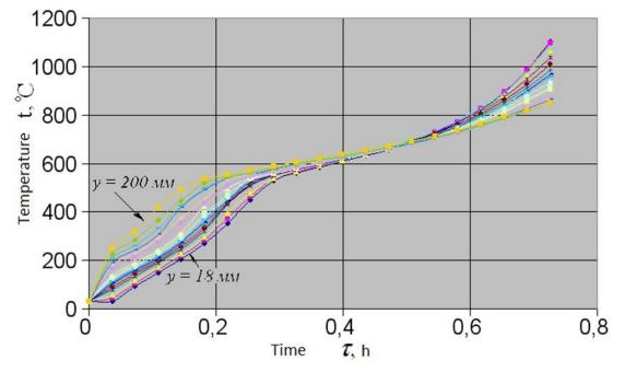
Figure 3. The results of the carbon bed temperature field simulation
