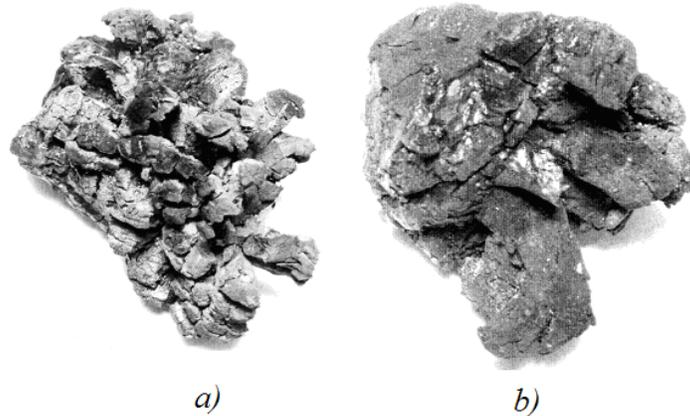
Figure 5. The reducing agent of Shubarkol coal; a - after thermo-oxidative coking; b - from the top of the ferroalloy furnace
