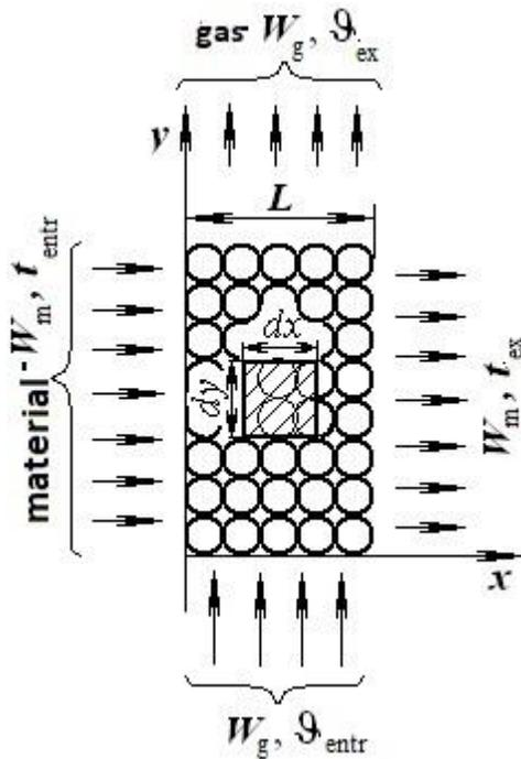
Figure 2. Scheme of heat exchange process in the layer of lump material
