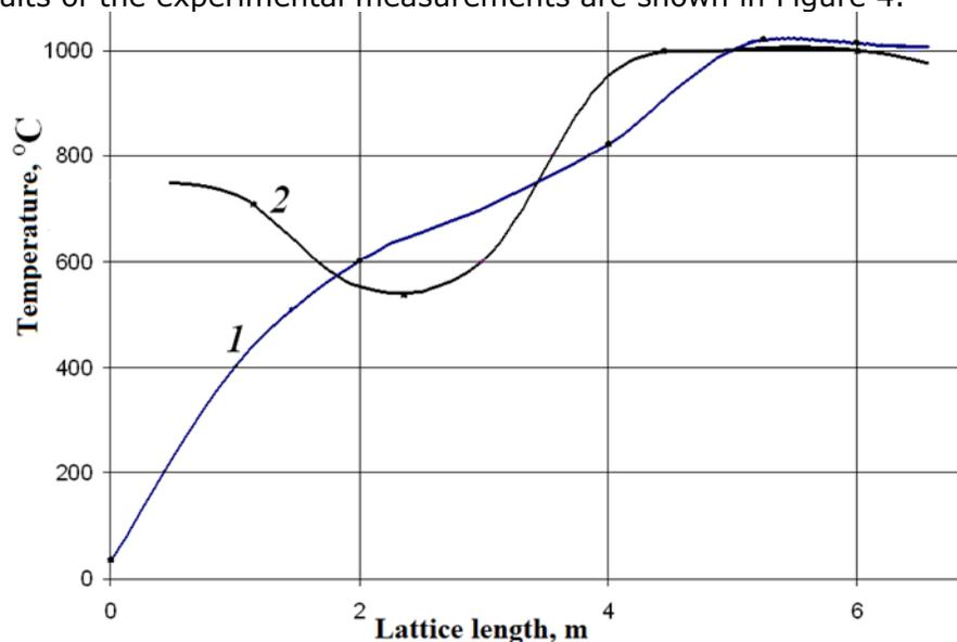
Figure 4. Temperature distribution along the lattice length; 1 - in the layer at a depth of 0.1 m (with a loading layer thickness of 0.2 m); 2 - in the furnace space at a height of 1
