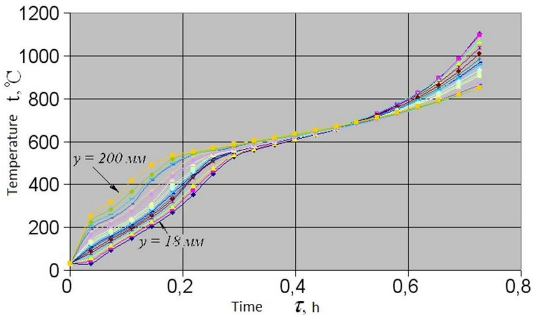
Figure 3. The results of the carbon bed temperature field simulation
