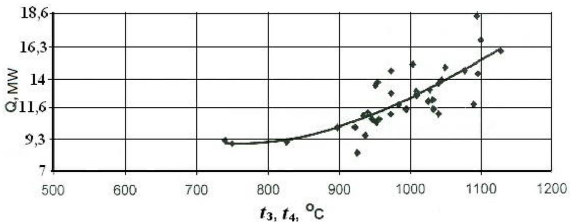
Figure 6. The dependence of the generated heat amount on the temperature in zones 3 and 4
