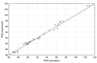
oline compounding model was evaluated by comparing the calculated octane mixing numbers with the experimental octane numbers determined for such flows as reformate (moving and stationary catalyst bed), isomerizate, alkylate, and catalytic cracking gasoline. The comparison results are presented in Fig. 2.
