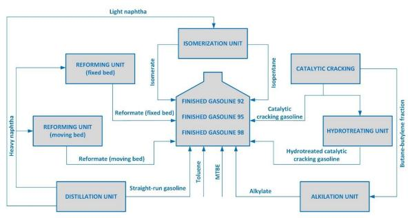
Figure 1. Scheme of the commercial gasoline production
