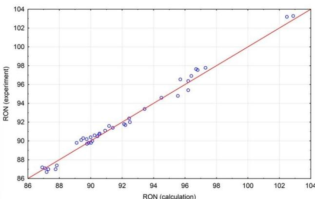
Figure 2. Verifying the calculation of octane mixing numbers
