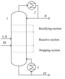
Fig. 1. Scheme of the reactive distillation column of methyl *tert*-butyl ether synthesis. I, II, III, IV – streams of isobutylene, n-butene, methanol and MTBE respectively; 1– reactive distillation column; 2 – condenser; 3 – reboiler.
