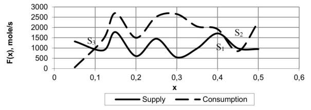
Fig. 3. Dependence of F<sup>supply</sup> and F<sup>consumption</sup> from methanol concentration in reactive section of the column
