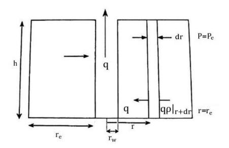
Figure 2. A cylindrical part of a hydrocarbon reservoir with length h (thickness of the reservoir) and thickness dr and inner radius r
