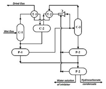
Figure 1. Low-temperature separation scheme
