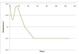
Figure 11. Temperature stabilization in second stage separator during certain time with half-opened valve
