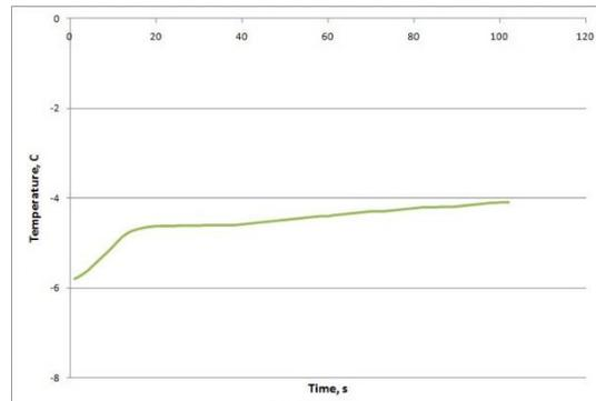
Figure 15. Temperature stabilization in second stage separator during certain time with quarter-opened valve
