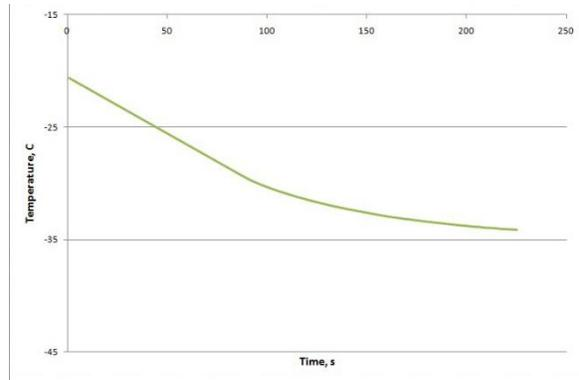
Figure 7. Temperature stabilization in second stage separator during certain time
