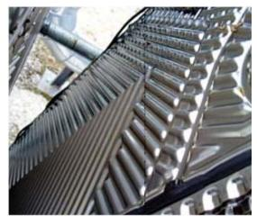
Picture 5 Cleaned warmth exchanging surface of the warmth exchanger
