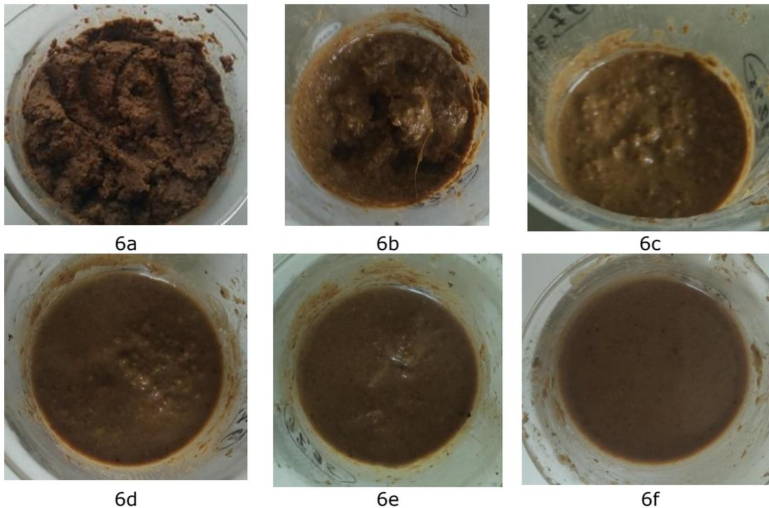
Figure 6. DS from external basin with different moisture content: a – 82,5 wt.%; b – 85 wt.%; c – 88 wt.%; d – 91 wt.%; e – 92 wt.%; f – 93 wt.%.
