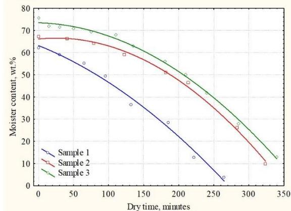
Fig. 8. Change in relative DS moisture content during thermal drying at a temperature = 150°C.
