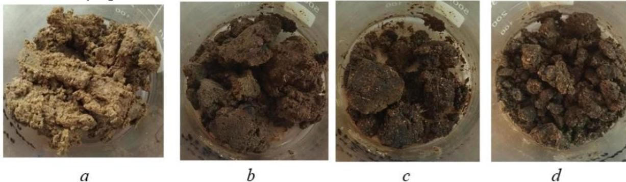
Fig. 7. DS during the drying process with changes in moisture content: a – 86,5 wt.%; b – 78,8 wt.%; c – 65,8 wt.%; d – 55,7 wt.%.
