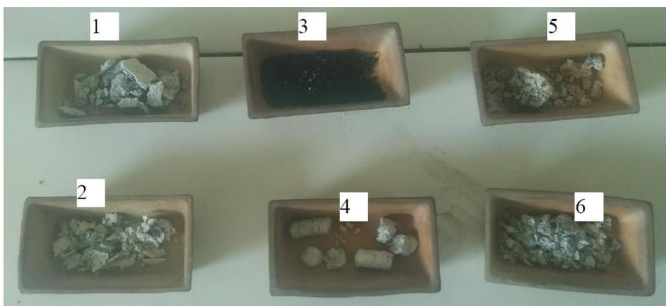
Fig. 9. DS ash: 1 - centrifuge feed (Artemivsk distillery); 2 - centrifuge fugate (Artemivsk distillery); 3 - DS after thermal drying (Artemivsk distillery); 4 - sunflower husk pellets; 5 - dregs from external DS-accumulation basin (Karavansk distillery); 6 - centrifuge feed (Karavansk distillery).
