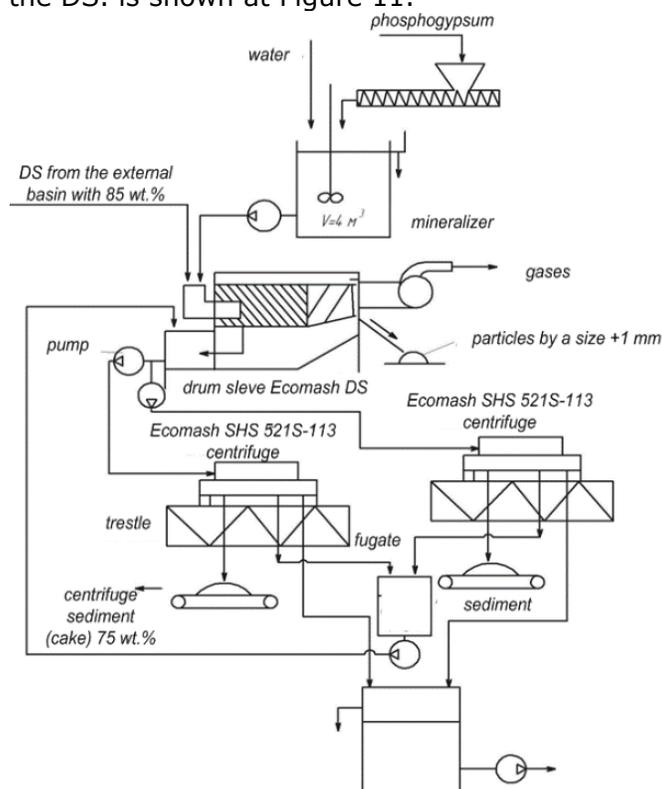
Fig. 11. Ecomash SHS 521S-113 centrifuges mechanical dewatering module (three-product mode) for DS.
