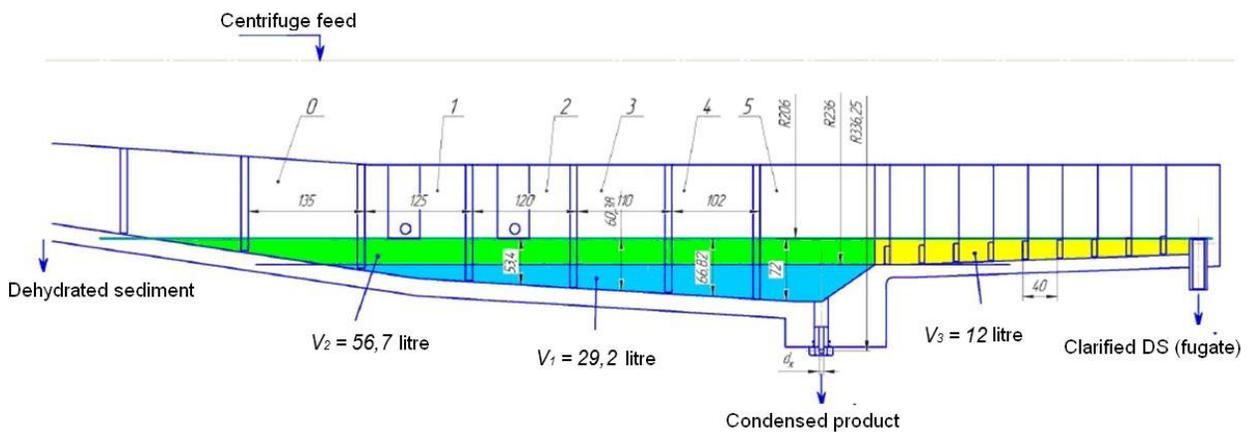
Figure 3. Longitudinal section of the Ecomash SHS 521 centrifuge rotor.
