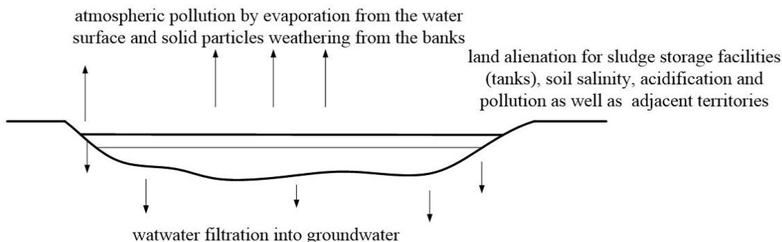
Fig 1. DS- accumulators basin negative environmental impact on ecosystem's components.
