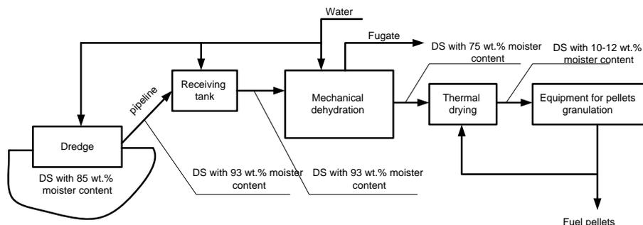
Fig. 10. Technological scheme for condensed DS processing into fuel pellets.
