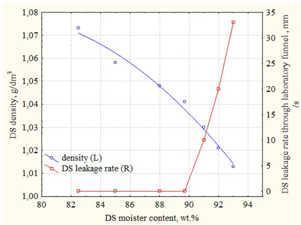
Fig. 5. DS dependence of change in density  $\rho$  and fluidity  $Q$  on moisture content  $W$ .
