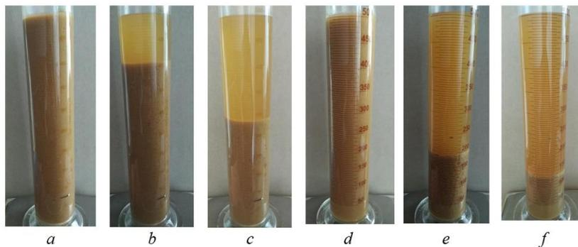
Fig 4. DS settling kinetics from centrifuge fed (dry matter concentration is about 49.25 g/L) and the fugate (dry matter concentration is about 27.25 g/L): a – initial DS; b – DS settling for 2 hours; c – DS settling for 20 hours; d – centrifuge fugate; d – fugate settling for 2 hours; e – fugate settling for 20 hours.
