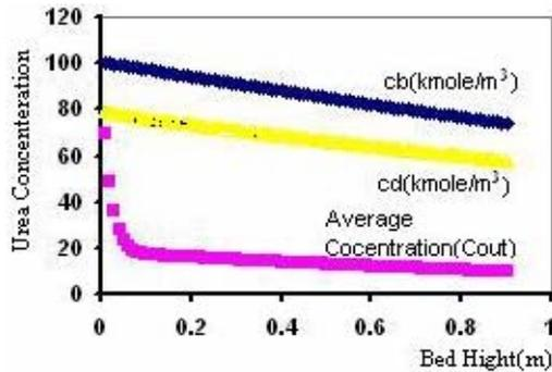
Fig(2)-Two phase model results: phase concentration profile (bubble , dense and average) and urea conversion vs. bed height;  $d_r=4.1\text{cm}$ ,  $u=.8\text{m/s}$ ,  $u_{mf}=.02344\text{m/s}$ ,  $k=13.7798$ ,  $n=.4$ ,  $T=380^\circ\text{C}$ ,  $D_e=.00001\text{m}^2/\text{s}^2$ ,  $H_{mf}=.5375\text{m}$
