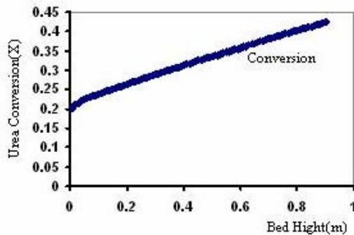
Fig(3)- Two phase model results: urea conversion vs. bed height;  $d_r=4.1\text{cm}$ ,  $u=.8\text{m/s}$ ,  $u_{mf}=.02344\text{m/s}$ ,  $k=13.4498$ ,  $n=0.4$ ,  $T=380^\circ\text{C}$ ,  $D_e=.00001\text{m}^2/\text{s}^2$ ,  $H_{mf}=.5375\text{m}$
