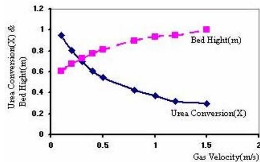
Fig(1)-two phase model results: urea conversion and bed height vs. gas velocity;  $u_{mf} = 0.0234 \text{ m/s}$ ,  $H_{mf} = 5375 \text{ m}$ ,  $D_r = 0.041 \text{ m}$ ,  $w = 400 \text{ g}$ ,  $emf = 425$ ,  $k = 13.7798$ ,  $n = 4$ ,  $D_e = 0.00001 \text{ m}^2/\text{s}$ ,
