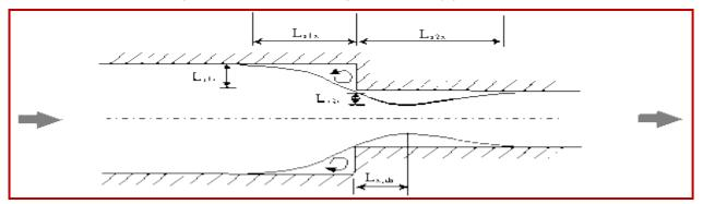
Figure 2. The upstream and downstream separations in the vicinity of the contraction
