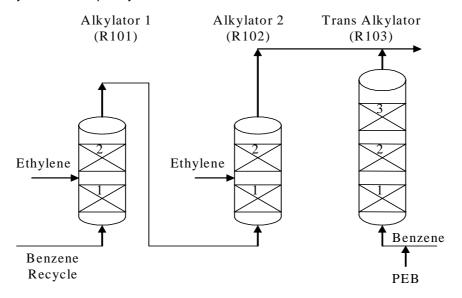
Fig.1- Simple Schematic of Ethyl Benzene Reactors
