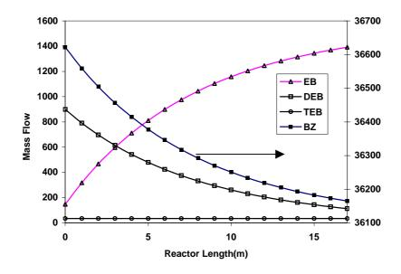
Fig. 5- Mass flow profile in R-103( kg / hr )
