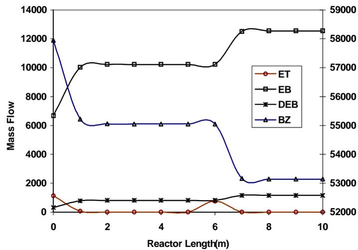
Fig. 4- Mass flow profile in R-102 ( $kg / hr$ )
