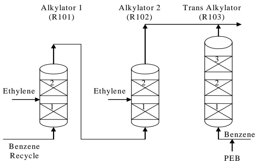
Fig.1- Simple Schematic of Ethyl Benzene Reactors
