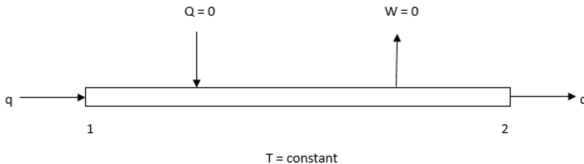
Figure 1. A gas transmission line model [5]
