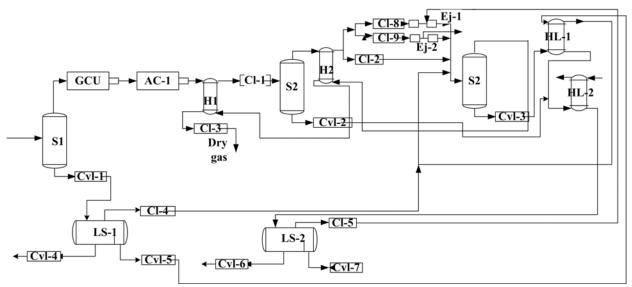
Figure 1. Technological scheme of gas treatment by low-temperature separation: S-1, S-2, S-3 - vertical gas separators; H1, H2 - heat exchangers such as "gas-gas", TL-1, TL-2 - type heat exchangers "liquid-liquid"; LS-1, LS-2 - three-phase separators - liquid separators; Cv-1, Cv-2, Cv-3, Cv-4, Cv-5 - control valves for gas; Cvl-1, Cvl-2, Cvl-3, Cvl-4, Cvl-5, Cvl-6, Cvl-7 - control valves for liquid; GCU - gas compressor unit - gas turbine; AC-1 - air cooler; Ej-1, Ej-2 - gas ejectors.
