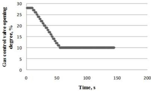
Fig. 3. Changes of gas control valve opening degree against time (manual control)
