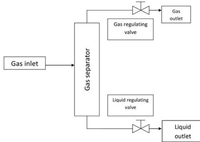
Figure 2. Schematic diagram of the gas first separation stage with valves of liquid level and pressure in apparatus control
