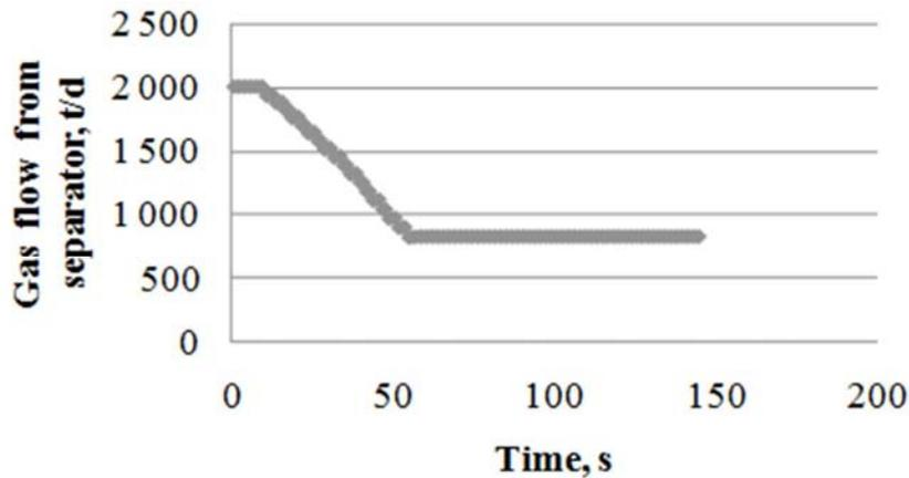
Figure 5. Gas flow rate from separator depending on time
