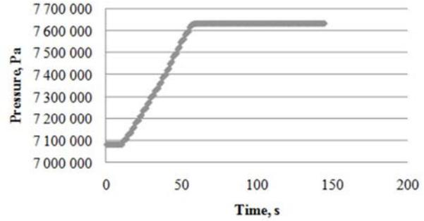
Fig. 4. Dependence of pressure in separator on time
