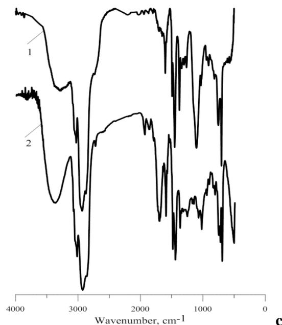
Fig. 1. The IR spectra of the initial resin (1) obtained by thermal (a), initiated (b), ionic polymerization (c); the modified resin (2) based on them (a, b, c) at the 0.5:1 «oxidative system:PR<sub>C9</sub> resin» component ratio
