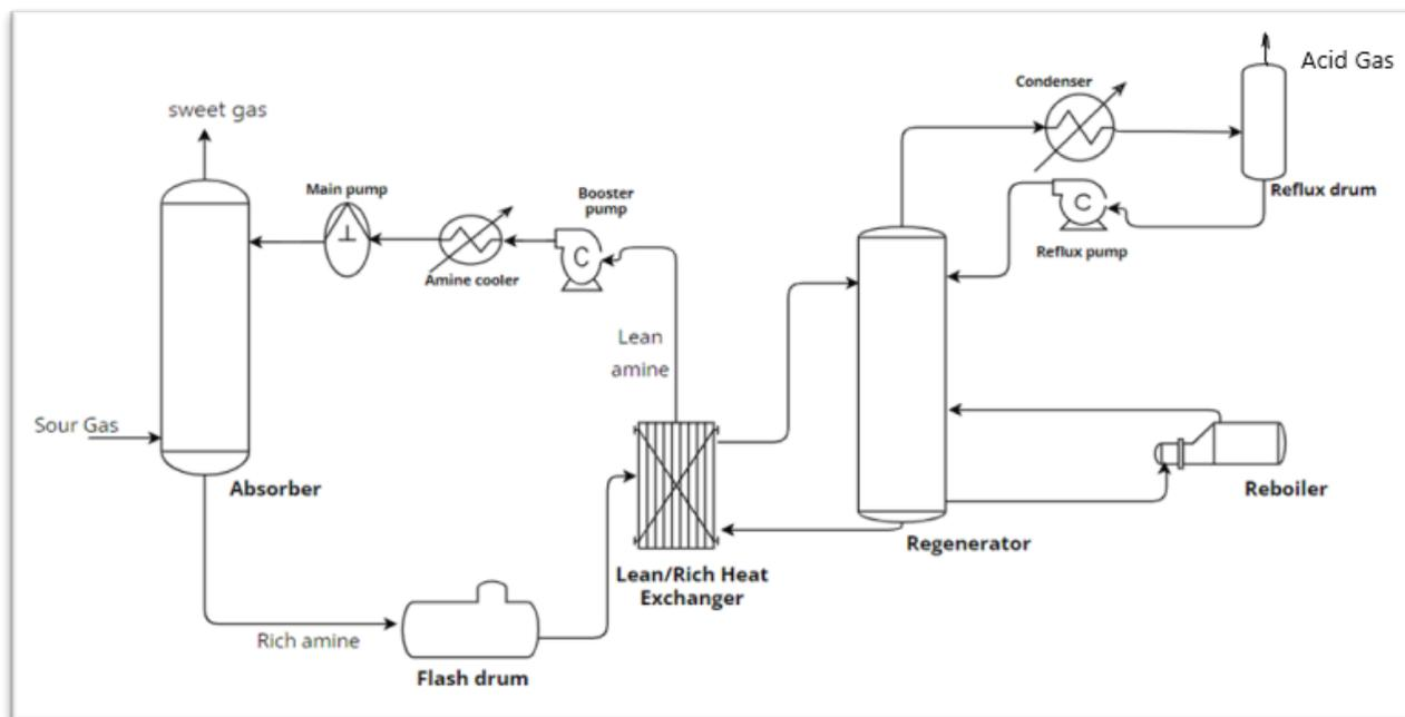
Figure 1. Typical gas sweetening plant PFD.
