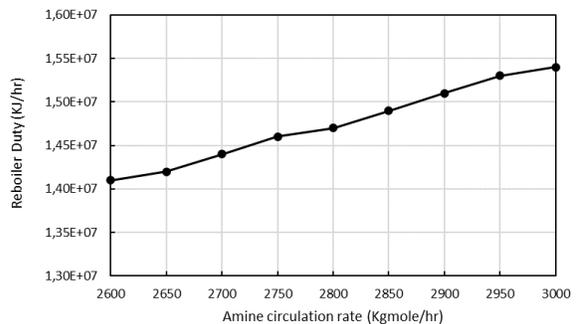
Figure 6- Effect of amine circulation rate on the reboiler duty.
