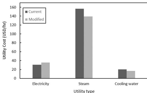
Figure 7. Utilities Cost comparison between the current and modified designs.
