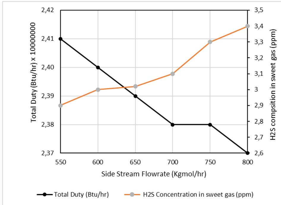
Figure 4. Effect of side stream flowrate on the total energy consumption and H<sub>2</sub>S concentration in the sweet gas.
