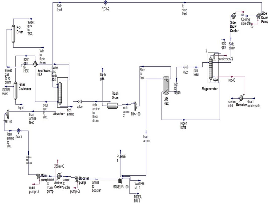
Figure 3. Simulation of the modified split-flow plant.
