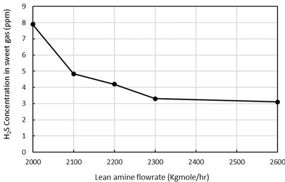
Figure 5. Effect of amine flowrate on H<sub>2</sub>S concentration in the sweet gas.
