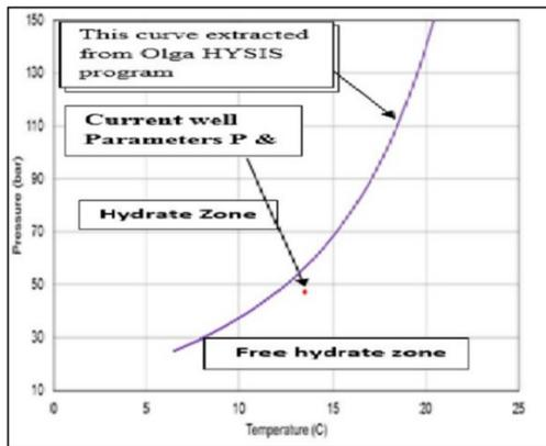
Figure 4. Hydrate curve for Well-51 free hydrate zone
