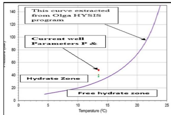
Figure 5. Hydrate curve for Well 59 inside hydrate zone
