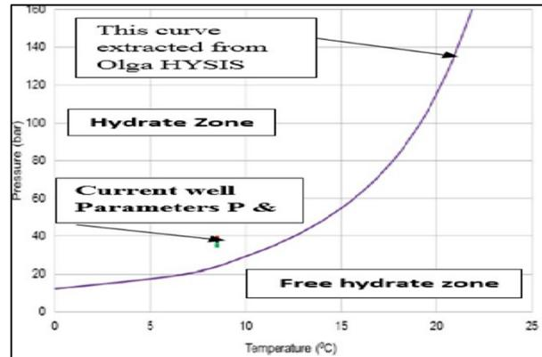
Figure 7. Hydrate curve for Well 24 inside hydrate zone.
