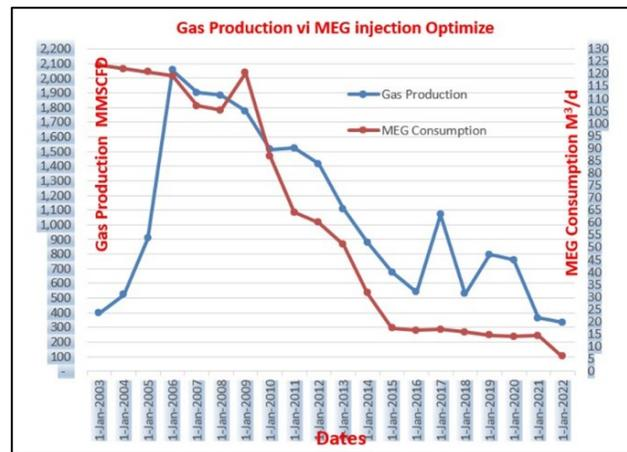
Figure 9. Gas production vs MEG injection
