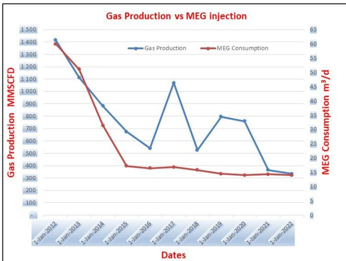
Figure 3. Actual case of deep marine gas plant MEG reduction
