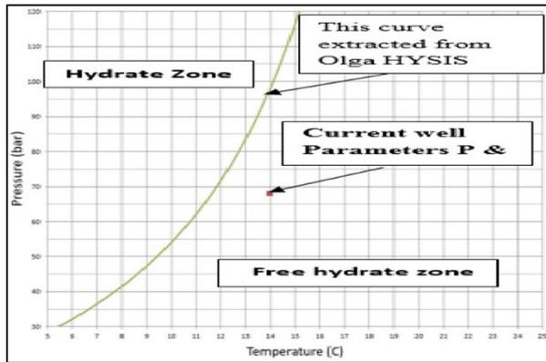
Figure 6. Hydrate curve for Well 37 free hydrate zone
