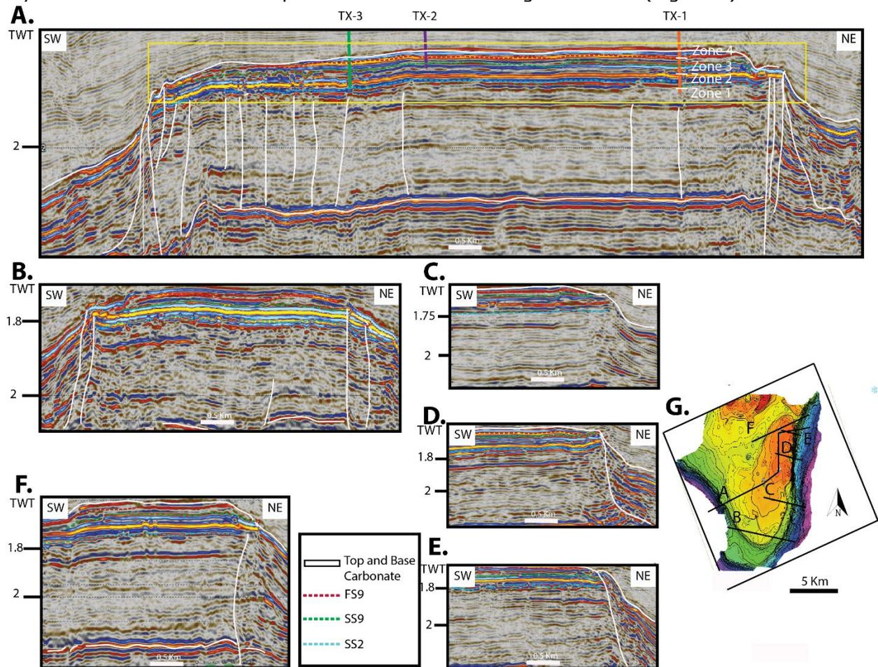
Figure 3. A. Arbitrary multiregional line interpreted northeast to southwest arbitrary covering the 3 study wells. B, C, D, E showing eastern arbitrary seismic lines showing the seismic character of the talus distribution and reef rim geometries. F. Arbitrary line displaying the seismic character of the Northern part of the build-up. G. The insert map shows the locations of the arbitrary lines
