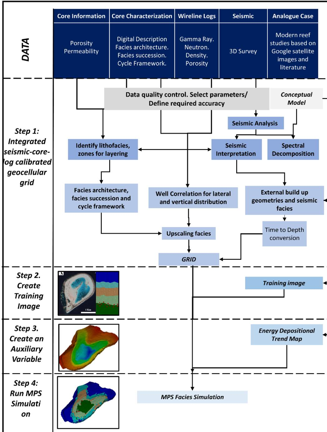
Figure 2. Proposed workflow methodology using MPS facies modelling. The basic data include geological information, seismic survey, well data and satellite images
