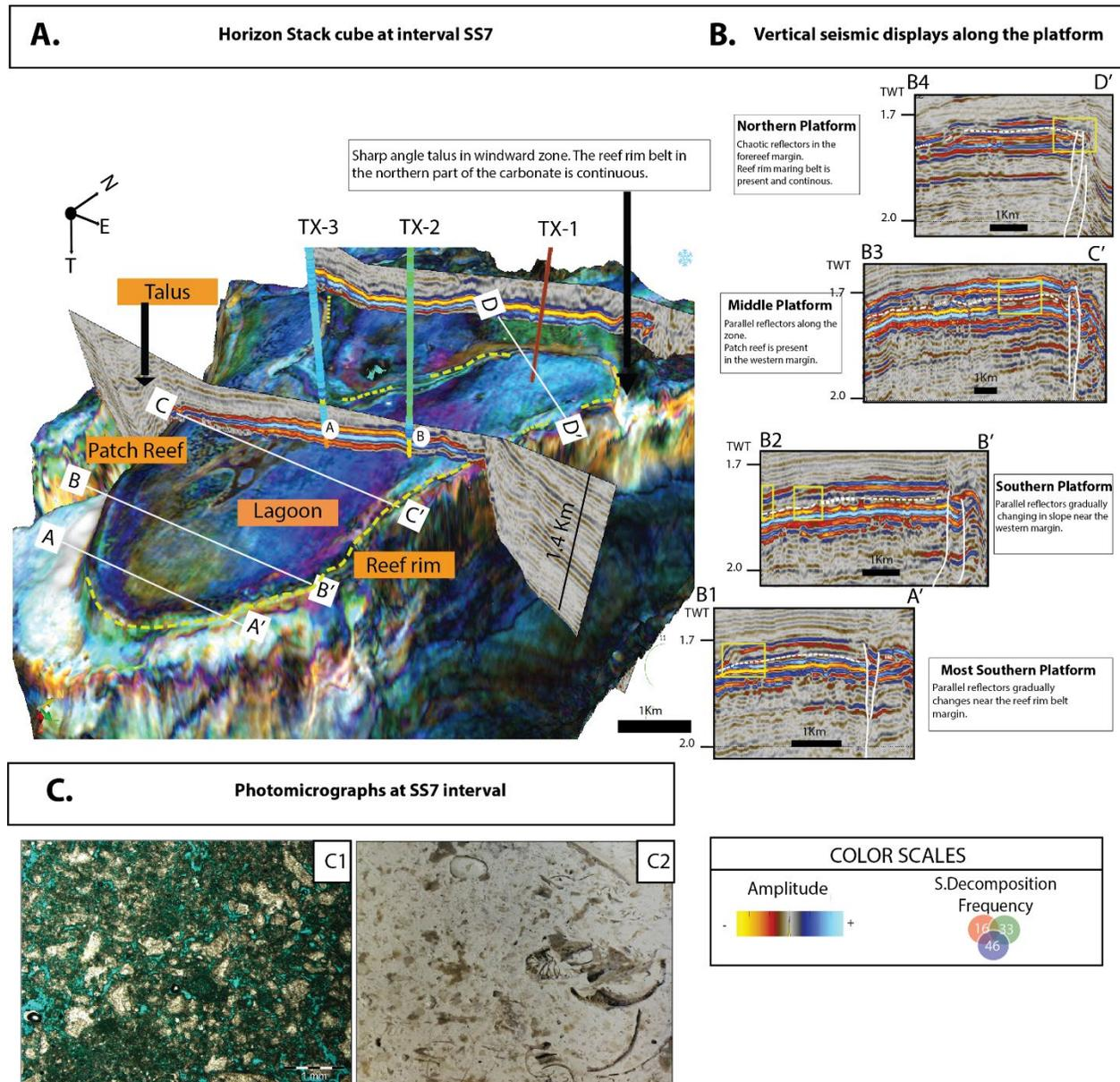
Figure 8. A. Cube display of SD attribute in horizon stack at SS7 interval B1, B2, B3, B4 Vertical seismic displays along with the platform where the less negative amplitude highlights the aggradational interval. C1, C2 Photomicrographs at SS7 interval with coral-dominated grainstone and coral-dominated floatstone with mouldic dominant porotypes and porosity of 28% and permeability of 42 Md
