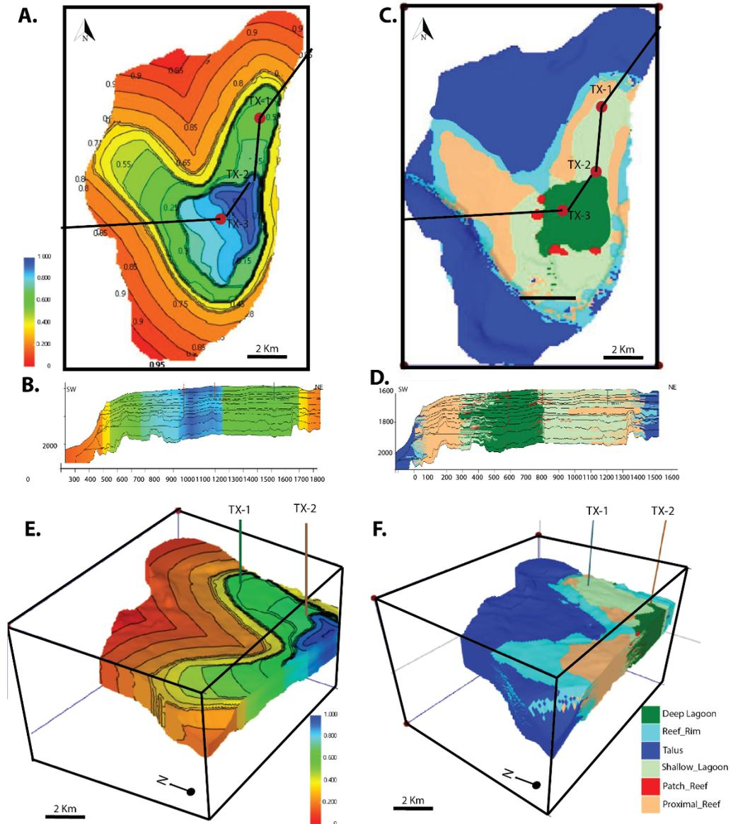
Figure 12. A. 3D energy trend model as an auxiliary variable for MPS simulation B. Northeast to the south-western cross-section of the energy trend map C. MPS 3D facies model of “TX” platform D. North-east to a south-western cross-section of the facies model. E. Western to Eastern cross-section of the 3D energy trend F. Western to Eastern cross-section of the 3D facies model
