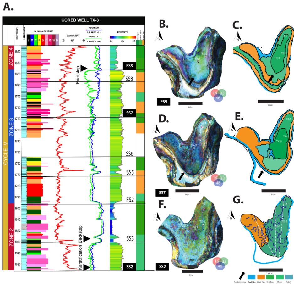
Figure 5. A. Well –Core-Seismic correlation of TX-3 well. The three selected intervals were used to define the trend maps for modelling. B, C correspond to FS9 is the Flooding interval with backstepping evidence in SD maps. D, E, corresponds to SS7 interpreted as an aggradational interval. F, G, corresponds to SS2 with a karst interval with dendritically pattern features
