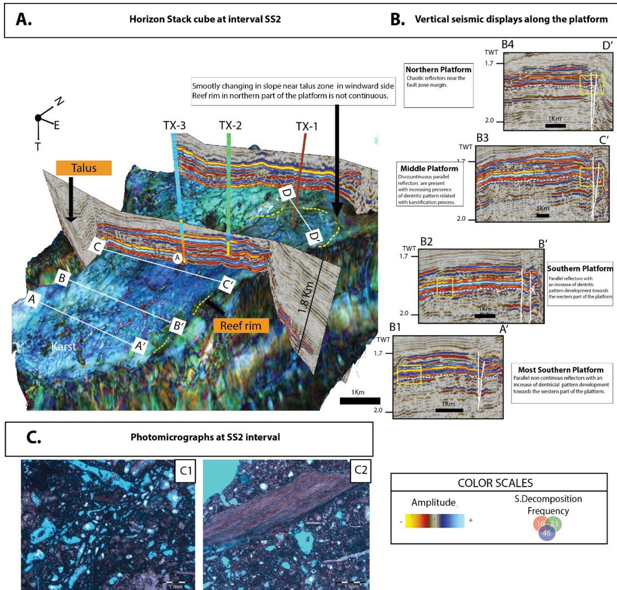
Figure 9. A. 3D Cube display of SD attribute in horizon stack at FS9 interval B1,B2,B3,B4E) Vertical seismic displays along with the platform where the most positive amplitude highlights the karst interval. C1, C2 Photomicrographs at SS2 interval with packstones to wackestones dominated facies with vuggy dominant poretype and porosity of 30% and average kh of 62 mD
