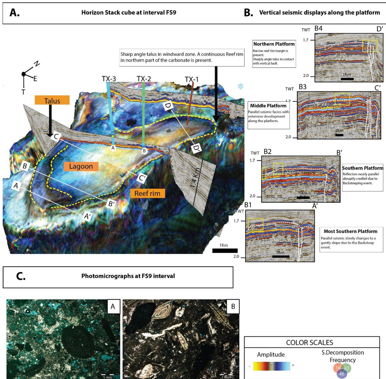
Figure 7. A. Cube display of SD attribute in horizon stack at FS9 interval B1, B2, B3 Vertical seismic displays along with the platform where the less negative amplitude highlights the flooding interval. C1,
