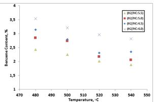
Figure 5. Effect of operating temperature on benzene content of the treated gasoline
