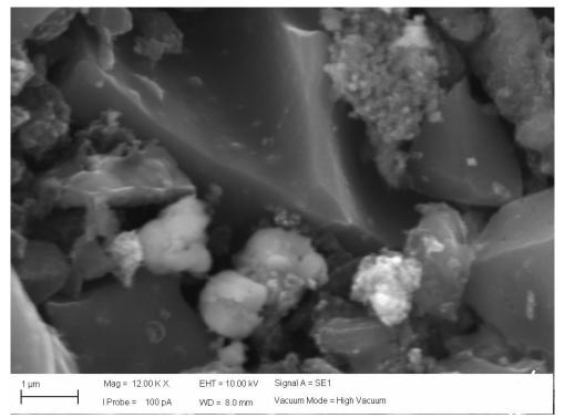
Figure 3. SEM image for fresh Ga-Re-Pt/Al<sub>2</sub>O<sub>3</sub> laboratory prepared catalyst sample
