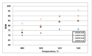
Figure 4. Effect of operating temperature on research octane number of the treated gasoline
