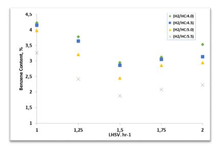
Figure 6. Effect of space velocity on benzene content of reformate
