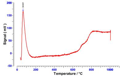
Figure 2. TPR for fresh Ga-Re-Pt/Al2O3 laboratory prepared catalyst sample
