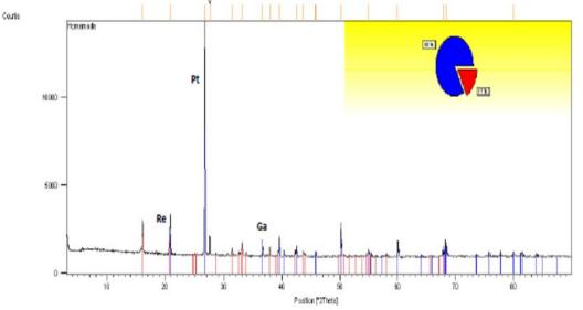
Figure 1. XRD patterns for fresh Ga-Re-Pt/Al $_2O_3$  laboratory prepared catalyst sample
