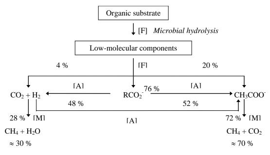
Figure 2 Skeleton drawing of the microbial creation of biogas. F – fermentation, A – acetogenesis, M – methanogenesis; percentage from <sup>[4]</sup>
