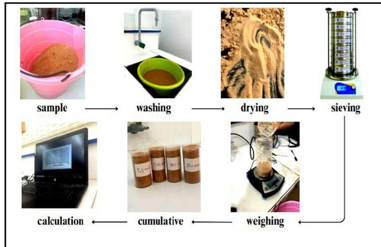
Figure 1. The used sample sand undergoes sequential preparation tests.
