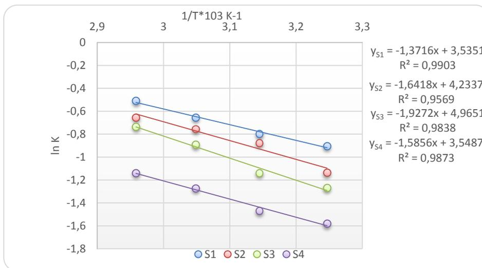
Figure 3. Variation of RT values of carbon steel with 3000ppm of (S<sub>1</sub>-S<sub>4</sub>) inhibitors at different temperatures
