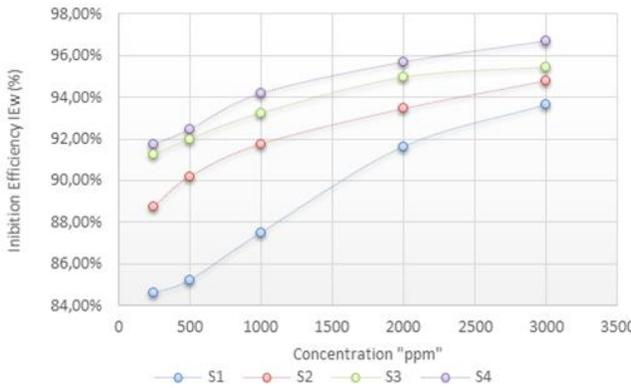
Figure 2. Variation of inhibition efficiency with different concentrations of the prepared inhibitors (S<sub>1</sub> – S<sub>4</sub>) in 0.5N HCl at 308K
