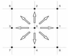
Figure 1.Lattice geometry and velocity vectors of the two-dimensional nine-speed D2Q9 model
