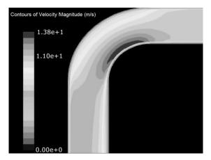
Figure 3. Contours of Velocity in considered bend
