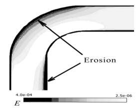
Figure 4. Contours of erosion mass parameter for considered bend
