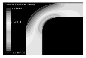
Figure 2. Contours of pressure in considered bend
