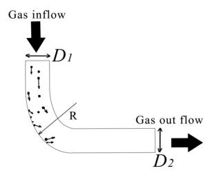
Figure 1. Schematic of bend and gas flow directions
