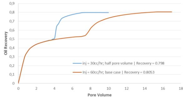
Fig. 9. Injection rate sensitivity with injection time
