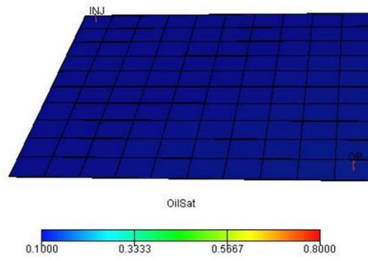
Fig. 15. Oil saturation map at the end of the ASP flood simulation
