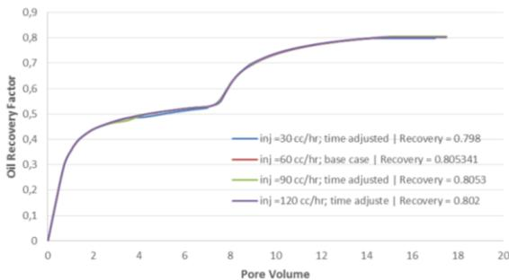
Fig. 8. Injection rate sensitivity with constant volume
