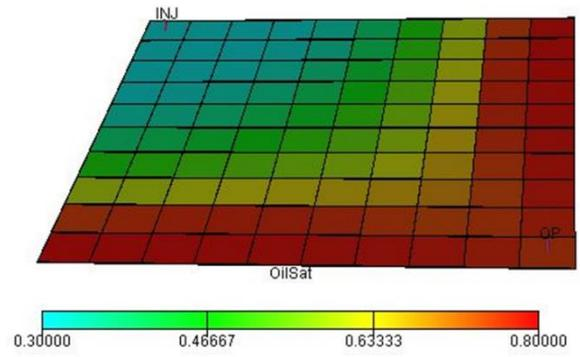
Fig. 13. Oil saturation map in the reservoir during the water flood simulation
