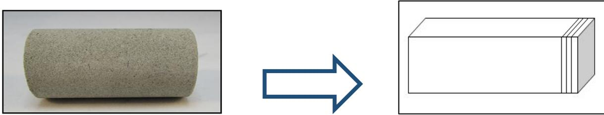
Figure 1. Scheme for approximating a cylindrical plug into cuboidal rock sample
