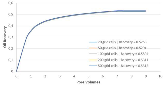
Fig. 7. Oil recovery variation with No of model grid cells
