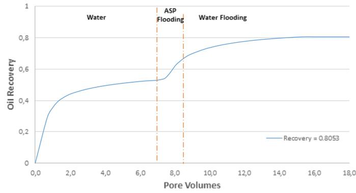
Fig. 8. Oil recovery for ASP flooding
