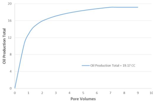
Fig. 6. Oil production total match for water flooding
