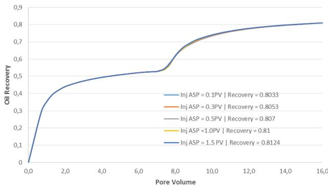
Sensitivity analysis on the pore volume of the ASP injected was carried out to identify the optimum value of ASP slug, which should be injected. With increasing pore volume of ASP slug injected, recovery factor also increased although the increase was very minimal (Fig. 11).
