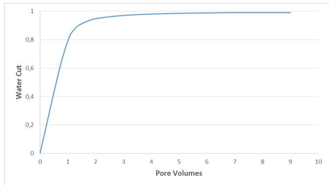
Fig. 5. Water cut match for water flooding
