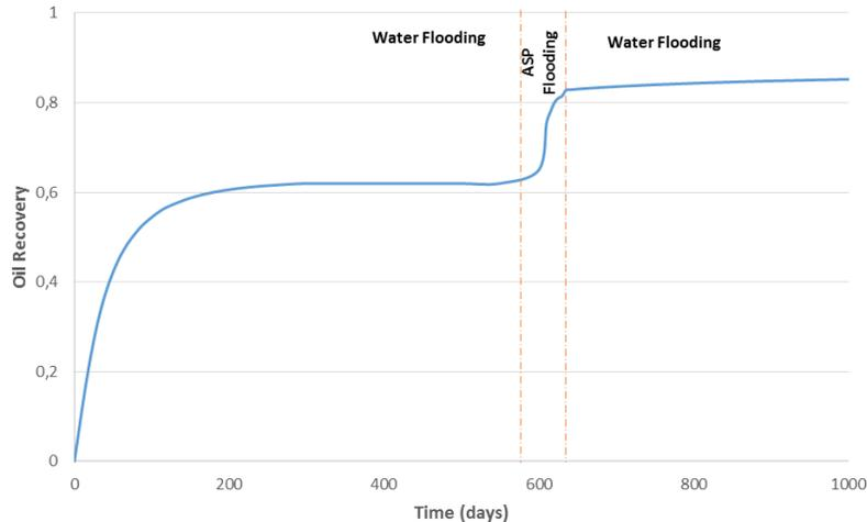
Fig. 16. Oil Recovery profile for ASP flooding of the synthetic reservoir
