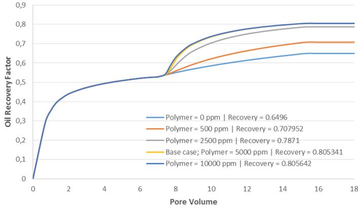
Fig. 10. Results of sensitivity analysis for polymer concentration
