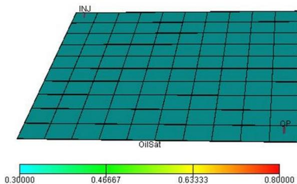
Fig. 14. Oil saturation map at the end of the waterflood simulation
