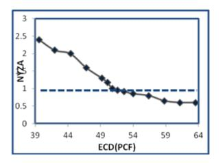
Figure9. NYZA versus ECD in Carbonate layers
