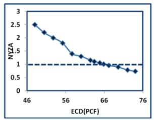
Figure 7. NYZA versus ECD in shale layers
