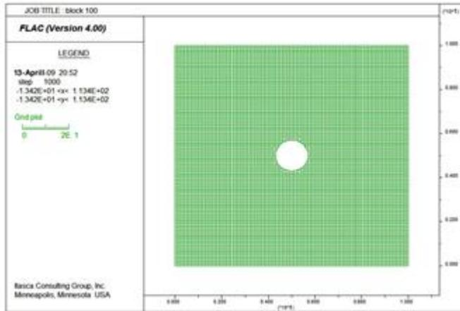
Figure 3. FLAC model created for a hole
