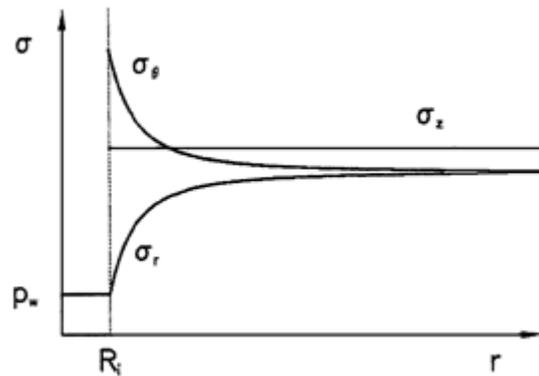
Figure 4. Stresses around a wellbore in a linear elastic formation [15]
