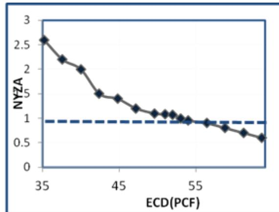
Figure 10. NYZA versus ECD in sandstone layers
