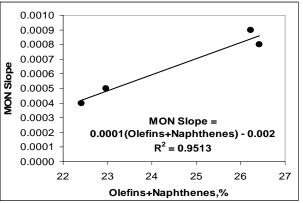
Figure 8 Dependence of the MON slope change on the upgraded gasoline total content of naphthenes and olefins
