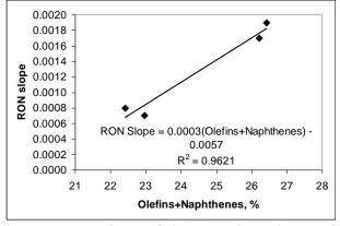
Figure 7 Dependence of the RON slope change on the upgraded gasoline total content of naphthenes and olefins
