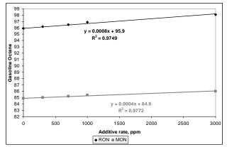
Figure 2 Dependence of octane number (RON, MON) on octane booster additive rate added to gasoline with RON = 95.9
