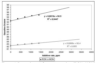
Figure 1 Dependence of octane number (RON, MON) on octane booster additive rate added to A-92 gasoline
