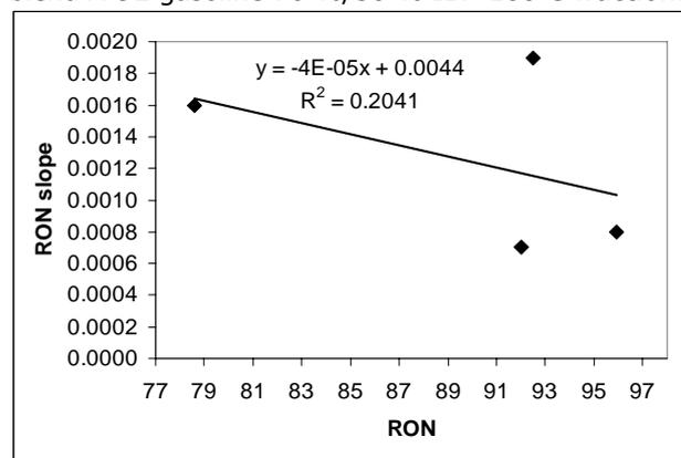
Figure 6 Dependence of the RON slope change on initial RON of the upgraded gasoline
