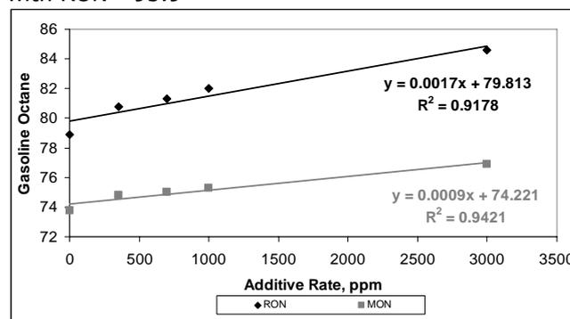
Figure 4 Dependence of octane number (RON, MON) on octane booster additive rate added gasoline blend A-92 gasoline 70 %/30 % IBP-100°C fraction.
