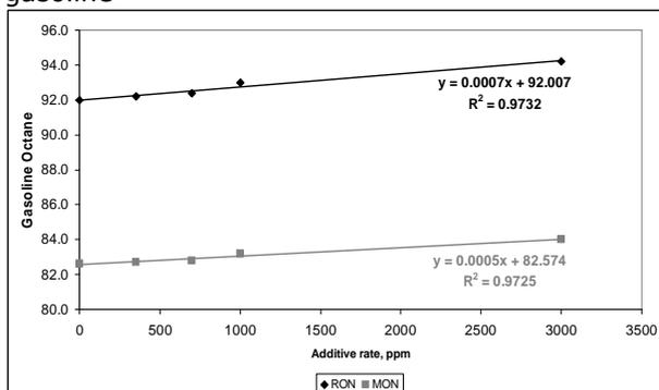
Figure 3 Dependence of octane number (RON, MON) on octane booster additive rate added to gasoline blend RON = 95.9 79 % / 21 % IBP- 100 °C fraction
