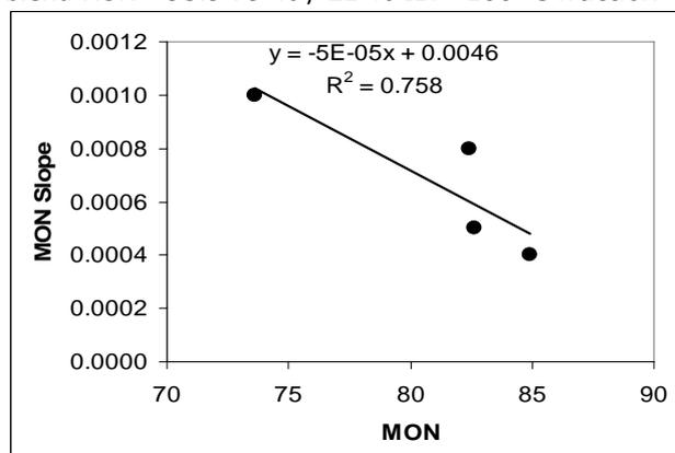
Figure 5 Dependence of the MON slope change on initial MON of the upgraded gasoline
