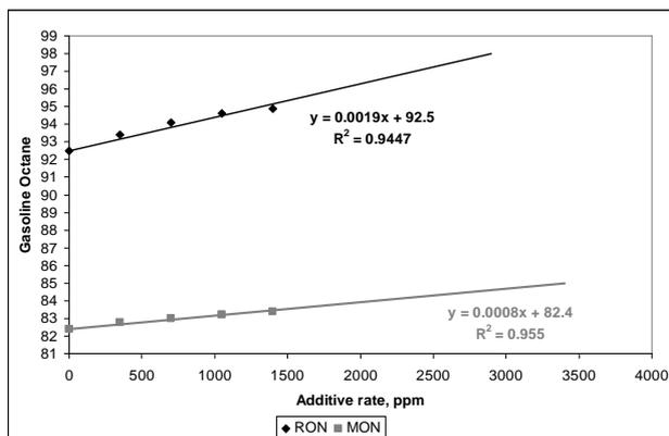
Figure 1 Dependence of octane number (RON, MON) on octane booster additive rate added to A-92 gasoline
