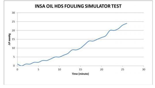
Fig. 2 Feed stock fouling simulator test
