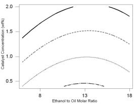
Fig. 3. Contour plots of ester yield vs. ethanol to oil molar ratio and catalyst concentration for the second-order model with reaction temperature of 57.5°C
