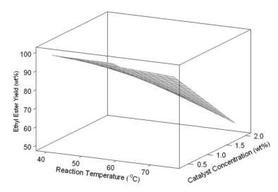
Figure 1. Response surface of ester yield vs. reaction temperature and catalyst concentration for the second-order model with ethanol to oil molar ratio of 12:1
