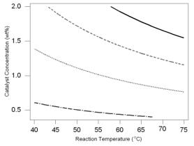
Fig. 2. Contour plots of ester yield vs. reaction temperature and catalyst concentration for the second-order model with ethanol to oil molar ratio of 12:1
