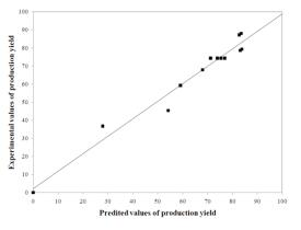
Figure 5. Comparison of experimental vs. predicted values of the ethyl ester production
