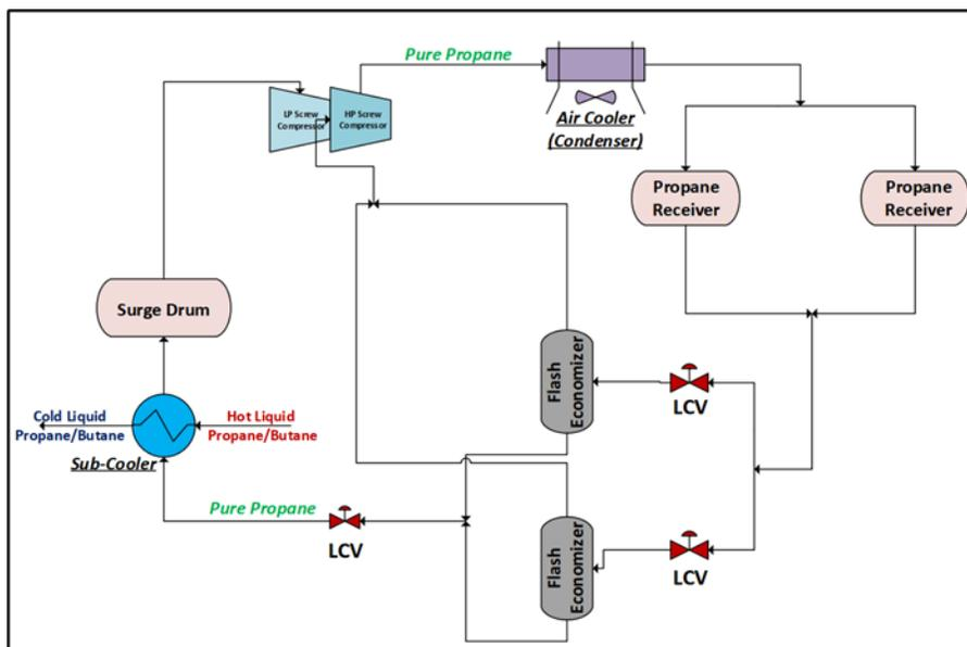
Figure 2. Pure propane refrigeration closed system.
