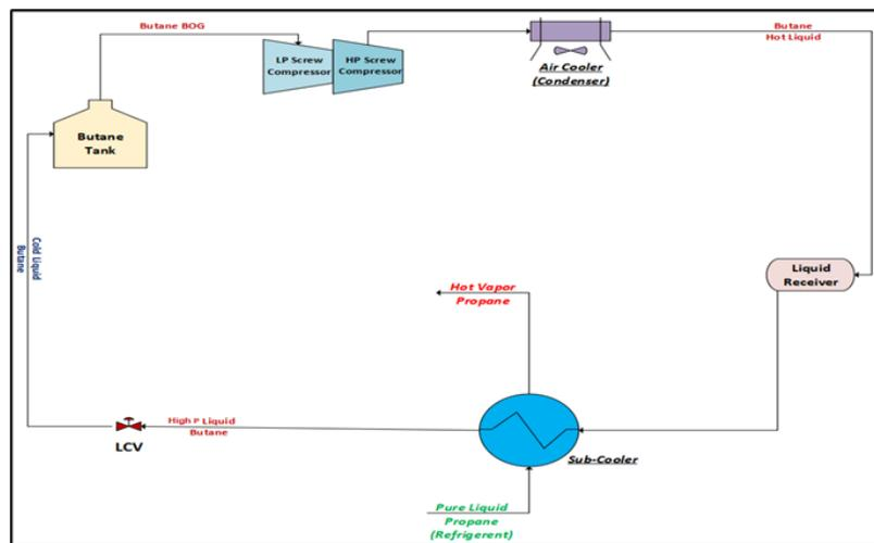
Figure 1. Butane BOG re-liquefaction process PFD.
