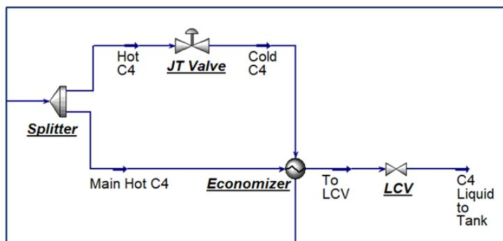
Figure 8. Splitting of butane mainstream using Aspen HYSYS.
