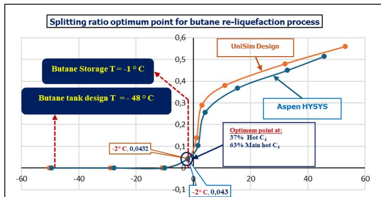
Figure 10. Optimum splitting point for the modified butane re-liquefaction process.
