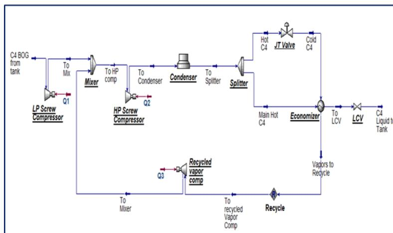
Figure 6. Simulation of the modified butane BOG (Aspen HYSYS).
