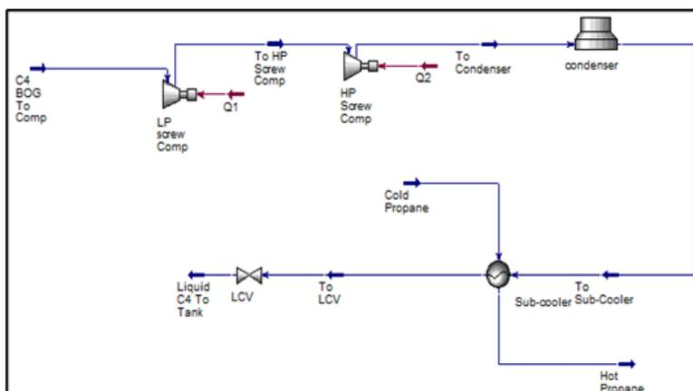
Figure 4. Simulation of the re-liquefaction process for butane BOG.
