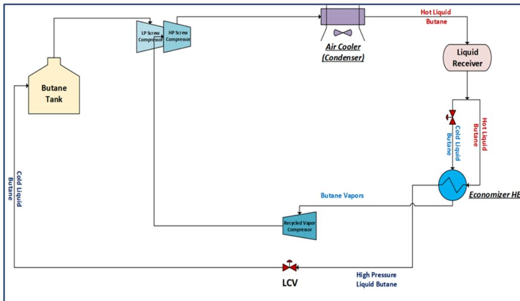
Figure 3. Butane BOG re-liquefaction process flow diagram.
