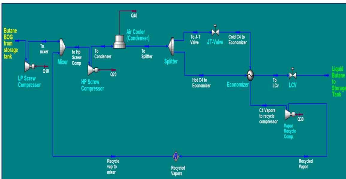
Figure 7. Simulation of the modified butane BOG (UniSim Design).
