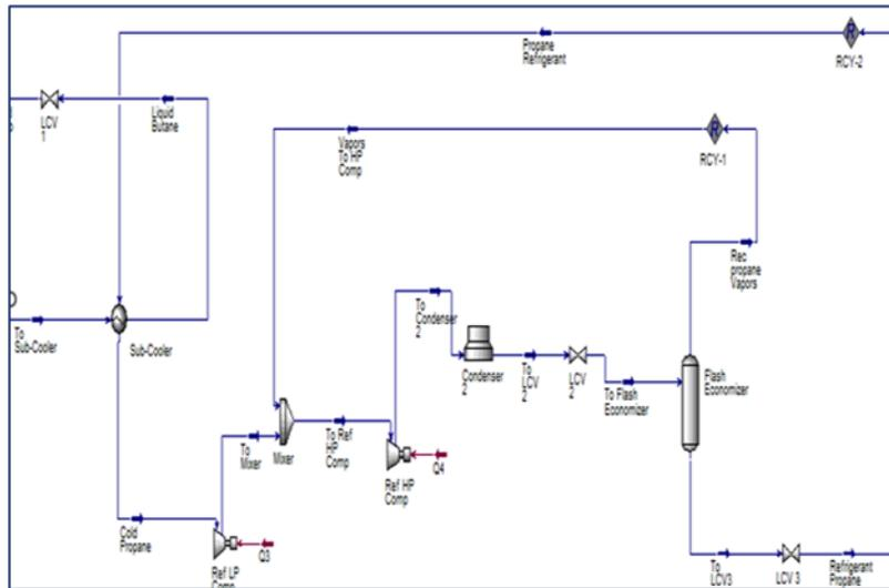
Figure 5. Simulation of the refrigeration closed system by Aspen HYSYS.
