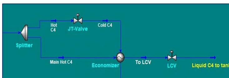
Figure 9. Splitting of butane mainstream using UniSim Design.
