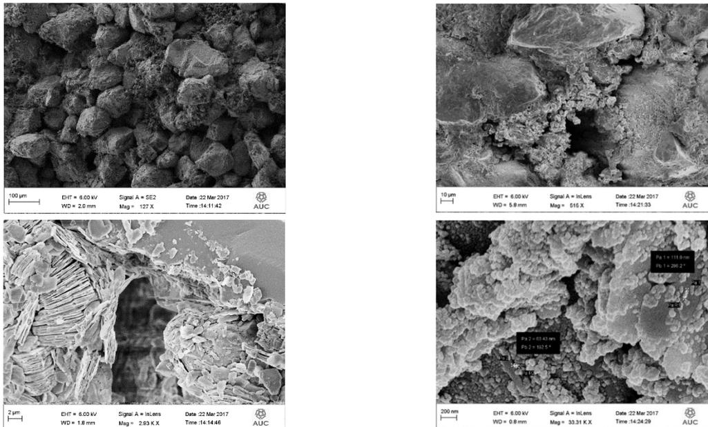
Fig. 1. (a) Clean rock sample before flooding (b) After the 5% wt. concentration nanofluid flooding.
