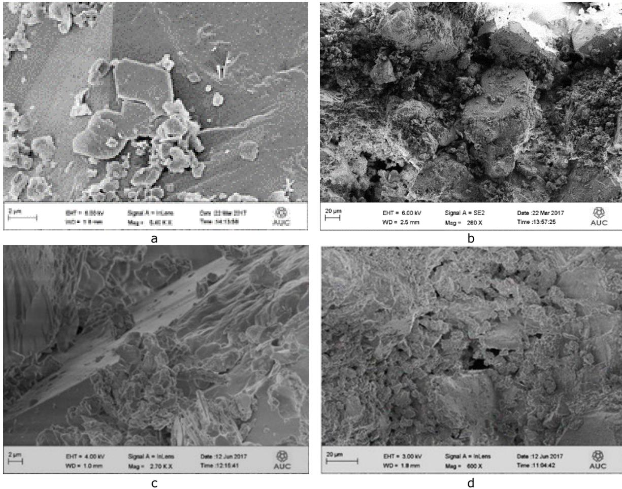
Fig. 6. (a) Clean rock sample before flooding (b) Rock sample after 0.2 PV 3% wt. concentration nanofluid (c) After 0.4 PV 3% wt. concentration nanofluid (d) After 0.6 PV 3% wt. concentration nanofluid.
