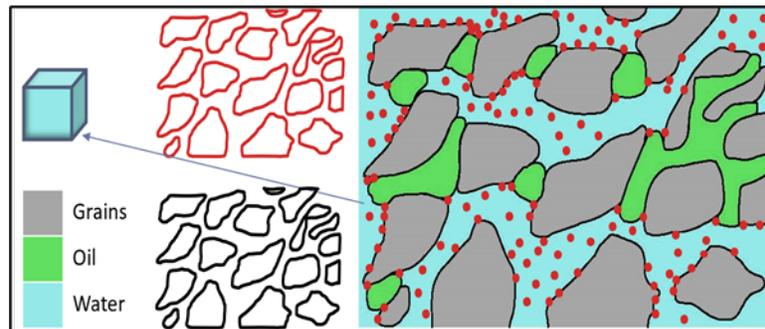
Fig. 10. Illustration of nanofluid critical volume in unit bulk volume of the pore system.
