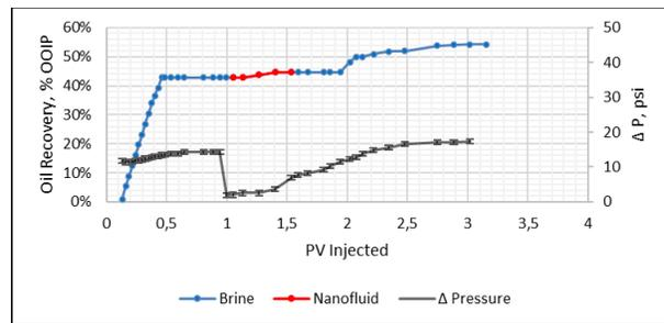
Fig. 4. LS nanofluid 3% - 0.4 PV slug size.
