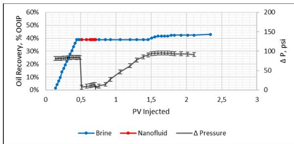
Fig. 3. LS nanofluid 3% - 0.2 PV slug size.
