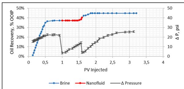
Fig. 5. LS nanofluid 3% - 0.6 PV slug size.
