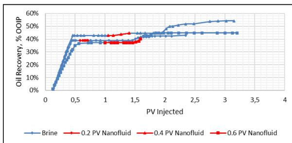
Fig. 7. LS nanofluid 3% - summary of PV slug size.
