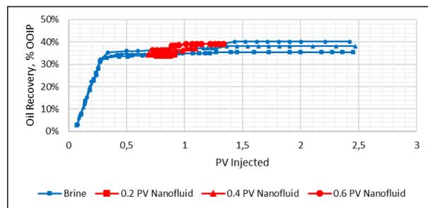
Fig. 8. LS nanofluid 1% - summary of PV slug size.
