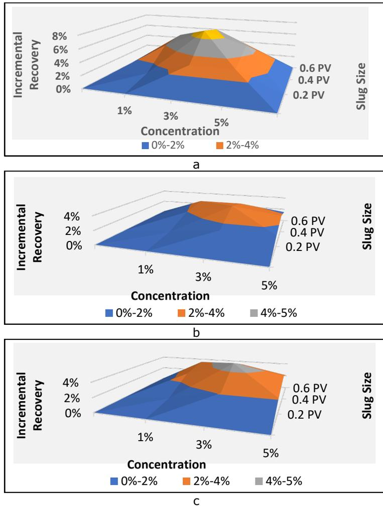
Fig. 9. Effect of nanofluid concentration and slug size (a) 0.2 CC/min (b) 0.1 CC/min (c) 0.4 CC/min.
