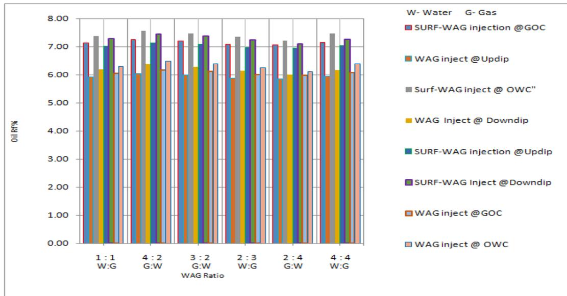
Fig 8. Plot of oil recovery factor against WAG ratio and fluid injection sequence for Obed oil rim reservoir
