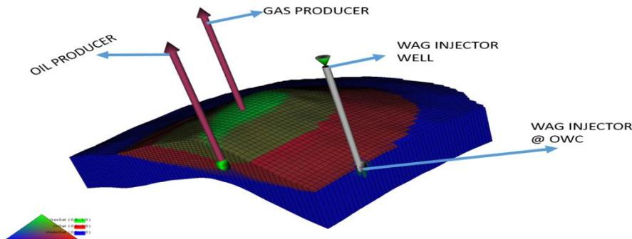
Fig. 3. 3D model view of concurrent development with injection well position at OWC for Obed field, Niger Delta
