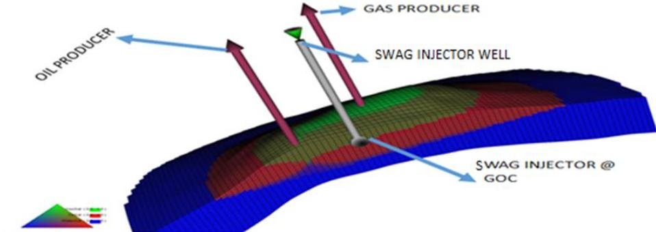
Fig. 2. 3D model view of concurrent development with injection well position at OGC for Obed field, Niger Delta, Nigeria
