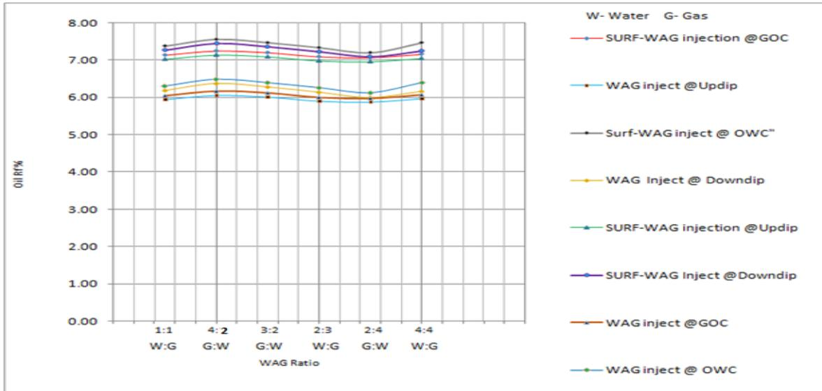
Fig. 5. Plot of oil recovery factor against fluids ratio and fluid injection sequence for various injection positions in concurrent development of Obed oil rim reservoir
