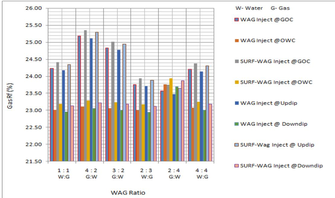
Fig. 7. Plot of gas recovery factor against fluid ratio and fluid injection sequence for Obed oil rim reservoir
