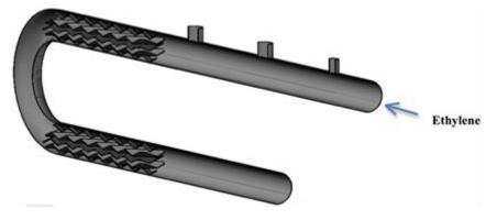
Figure 1. Model of the mixing chamber in longitudinal section
