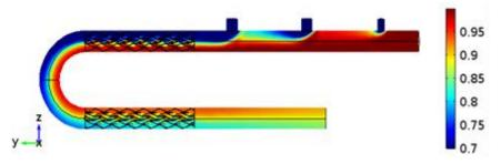
Figure 3. Volume fraction of ethylene at second option (t = 2 sec)
