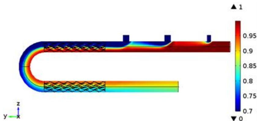
Figure 2. Volume fraction of ethylene at first option (t = 2 sec)
