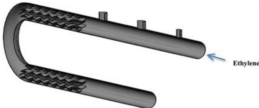
Figure 1. Model of the mixing chamber in longitudinal section
