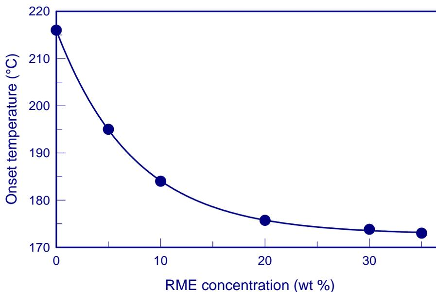
**Figure 6** Oxidation stability of biodiesel fuel by PDSC technique
