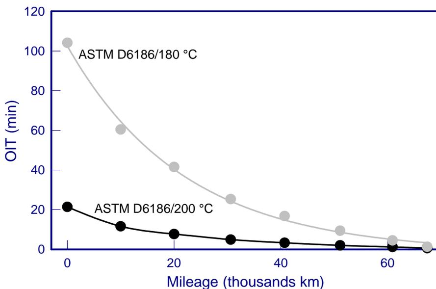
**Figure 3** Decrease of OIT of motor oil during operation in a heavy-duty engine Volvo FH12
