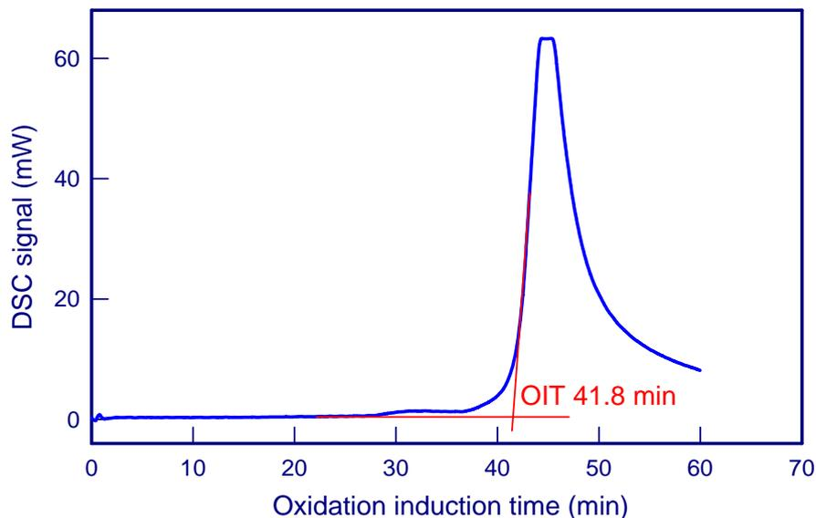
**Figure 1** Pressure DSC analysis of engine oil
