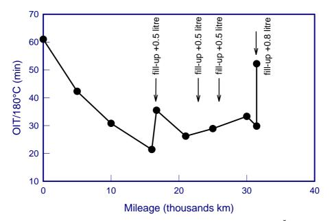
Figure 4 Decrease of OIT of motor oil during operation in a personal car Škoda Octavia 1.9 TDi (diesel fueled)
