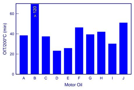
Figure 2 Oxidation stability of SAE 5W-30 motor oils by PDSC
