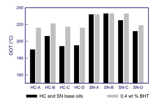
Figure 5 Oxidation stability of some HC and SN oils and effect of the BHT antioxidant
