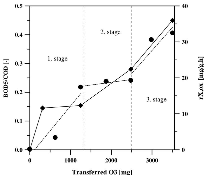
**Figure 4.** Relation of BOD<sub>5</sub>/COD (◆) and specific exogenous respiration rate (●) from transferred O<sub>3</sub> during MBT ozonation
