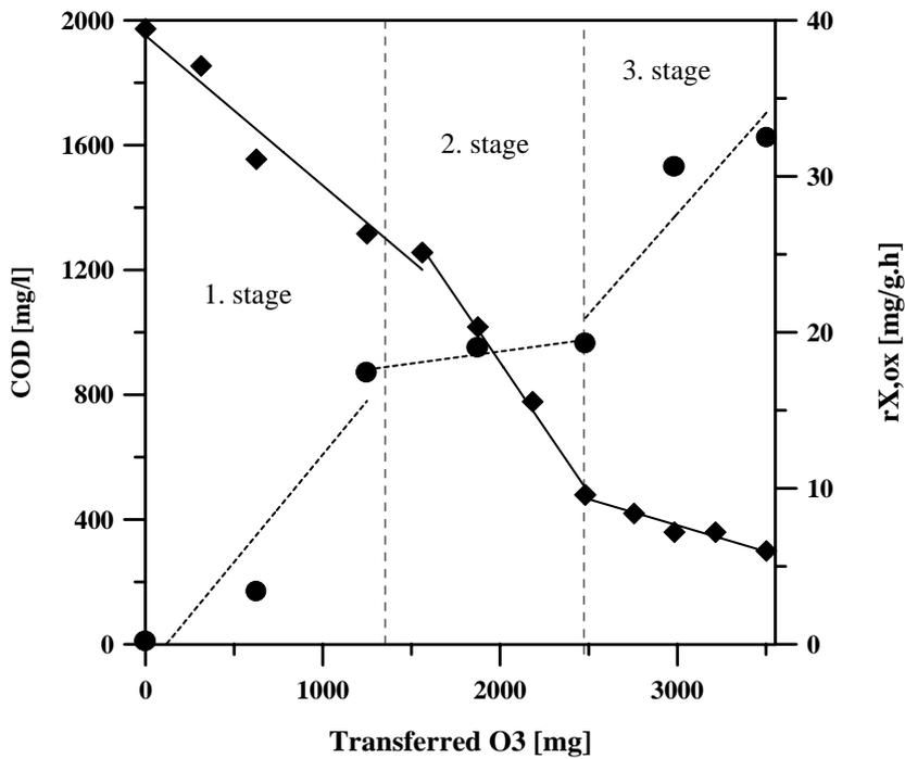
**Figure 3.** Modification of respiration activity of activated sludge (●) during ozonation of MBT solution in comparison with decrease of COD values (♦)
