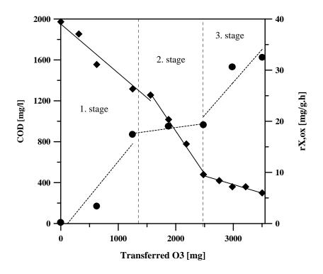
**Figure 3.** Modification of respiration activity of activated sludge (•) during ozonation of MBT solution in comparison with decrease of COD values (•)
