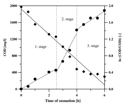
Figure 2. Experimental (\*) and calculated (solid line) time dependencies of COD during ozonation
