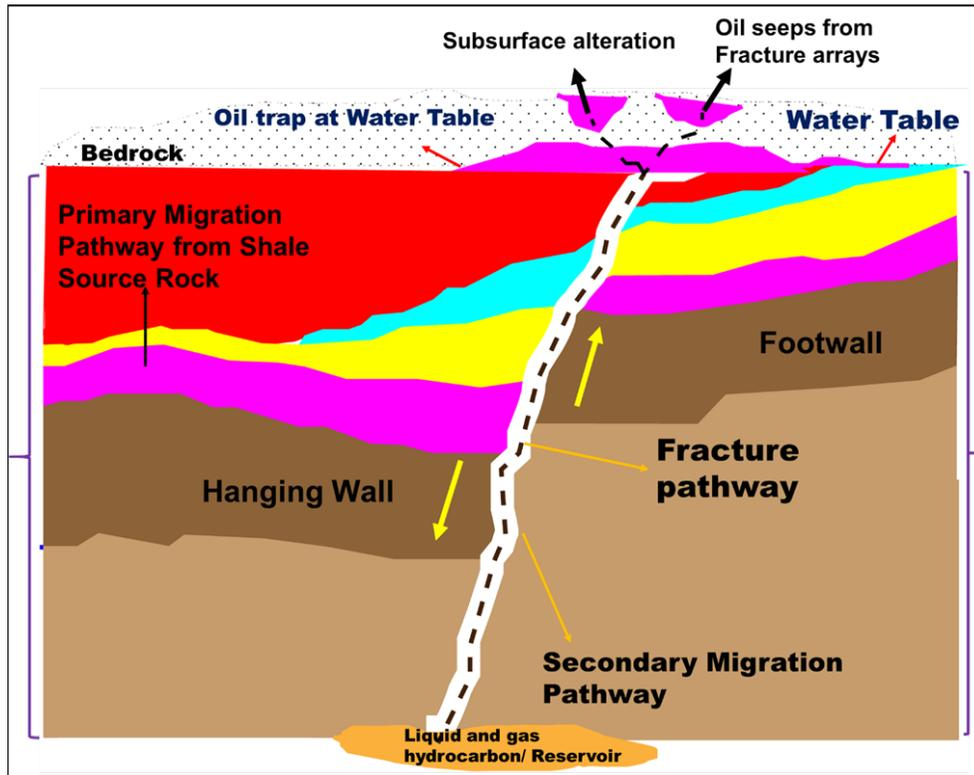
Fig. 7. Normal fault system of the Nsukka Formation of Anambra Basin showing schematic design of fracture pathway, seepage processes and dispersal mechanisms at Ikpankwo quarry.
