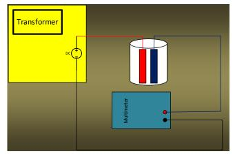
Figure 2. The laboratory set-up used for the measurement of crude oil conductivity
