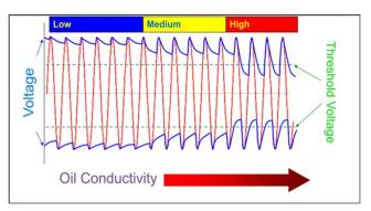
Figure 1.Voltage decay as a function of increased crude oil conductivity [9]
