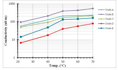
Figure 3. Electrical conductivity of the crude oils versus temperature
