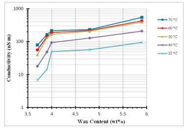
Figure 4. Electrical conductivity of the crude oils versus wax content
