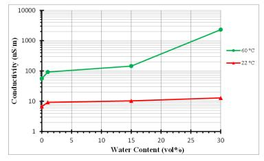
Figure 5. Electrical conductivity of w/o emulsion versus water content for crude "D"
